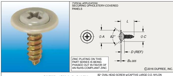
PART NO. EXAMPLE: OHCWL 4SM 6 D S42GY = WASHER, SHEET METAL, 4-24 X 3/8" LG, STEEL, PHILLIPS DRIVE, SEMI-GLOSS GRAY PER FED-STD-595 NO. 26622
