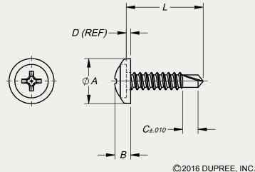
PART NO. EXAMPLE: DPSW 10SMB 10 ZR S04GN = PAN-L-SCREW, SHEET METAL, DRILL POINT 10-16 X 5/8" LG, STEEL, RoHS ZINC, PHILLIPS DRIVE, SEMI-GLOSS GREEN PER FED-STD-595 NO.24300
