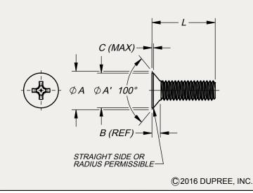
PART NO. EXAMPLE: **FH** 10**F** 6 ZR S01YE = 100° FLAT HEAD SCREW, .190-32 X 3/8" LG, STEEL, RoHS ZINC, PHILLIPS DRIVE, SEMI-GLOSS YELLOW PER FED-STD-595 NO. 26555
